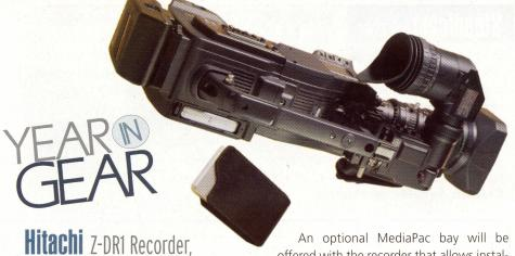
Hitachi Denshi America's tapeless Z-DR1 recorder docks to the company's Z-series professional camera models, enabling the cameras to be used handheld and in the field. The Z-DR1 records to removable MediaPac hard disk drive media, available in capacities from 20GB to 120GB. The digital recording compression is 25Mb/s; file
